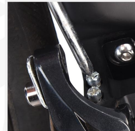
When shifting, if the chain has been separated from the internal test pinion, L should rotate clockwise. If the chain has to be separated from the external large cog, H should be turned clockwise
