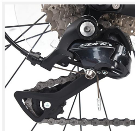
The rear derailleur - Frequent use, regular lubrication and maintenance
