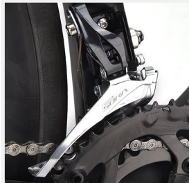
The H & L adjustment bolt of front derailleur
